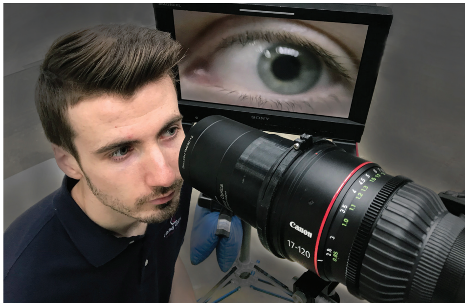
Shot with Canon Cine-Servo 17-120 and a +3 and +2 Brilliant Macros combined, using our stacking adapter.
